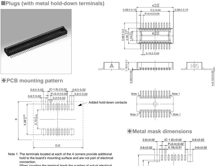
When counting the terminal leads the number of actual electrical circuits is lower by 4. Example: Connector with 24 terminal leads will have 20 actual electrical connections when mated with corresponding part.
